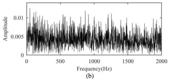
Fig. 10. Time domain waveform and envelope spectrum of bearing vibration signal. (a) Time-domain waveform; (b) Envelope spectrum.
