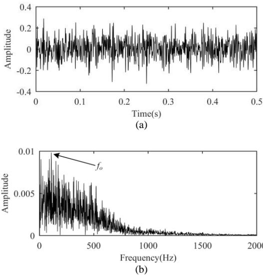
Fig. 12. Time domain waveform and envelope spectrum of reconstructed vibration signal. (a) Time-domain waveform; (b) Envelope spectrum.
