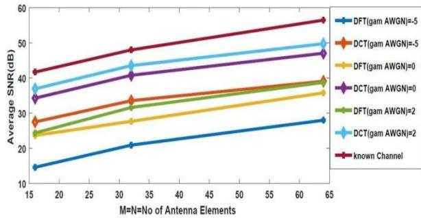
Fig 9. 2DFT Vs 2D DCT Method: Average SNR (dB) Vs No of antenna elements.
