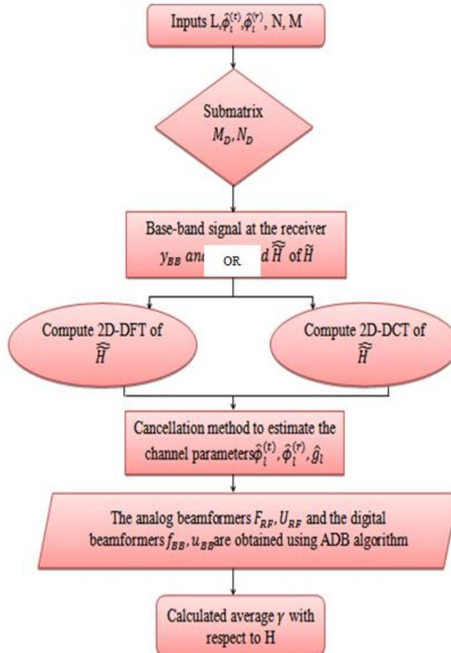
Fig.5. 2D-DCT based channel estimation
