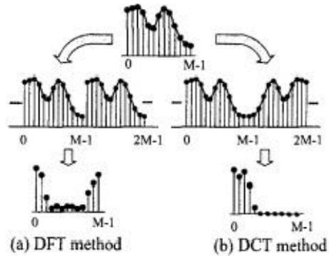
Fig. 4. Comparison between DFT and DCT Method
