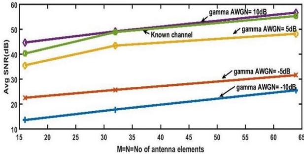
Fig 8. 2DFT Method: Average SNR (dB) Vs No of antenna elements
