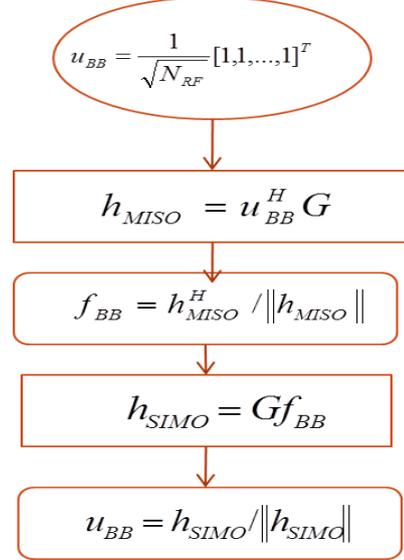
Fig. 7. Analog digital beamforming
