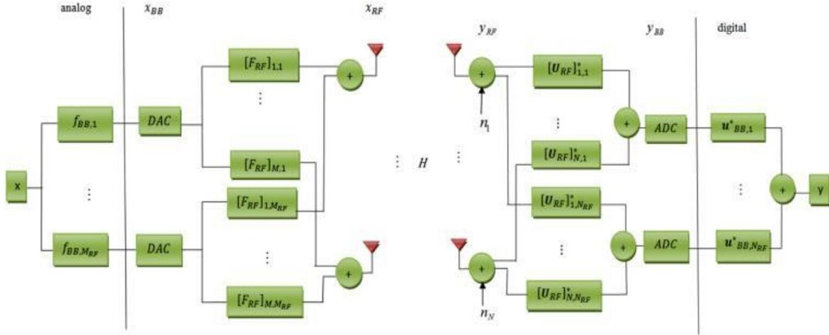
Fig. 3. Fully connected Hybrid beamforming architecture
