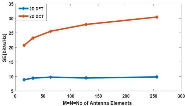
Fig. 10. Spectral efficiency Vs No of elements
