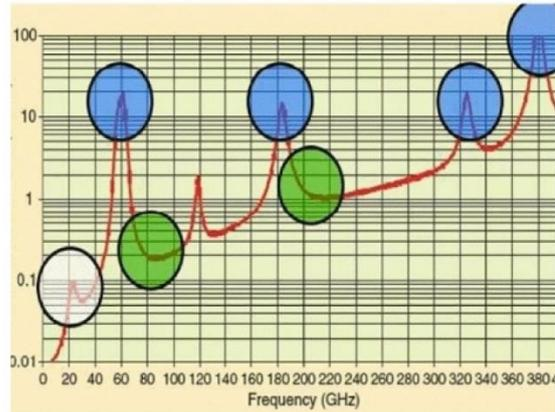
Fig. 1. Atmospheric absorption of electromagnetic waves [7–8]
