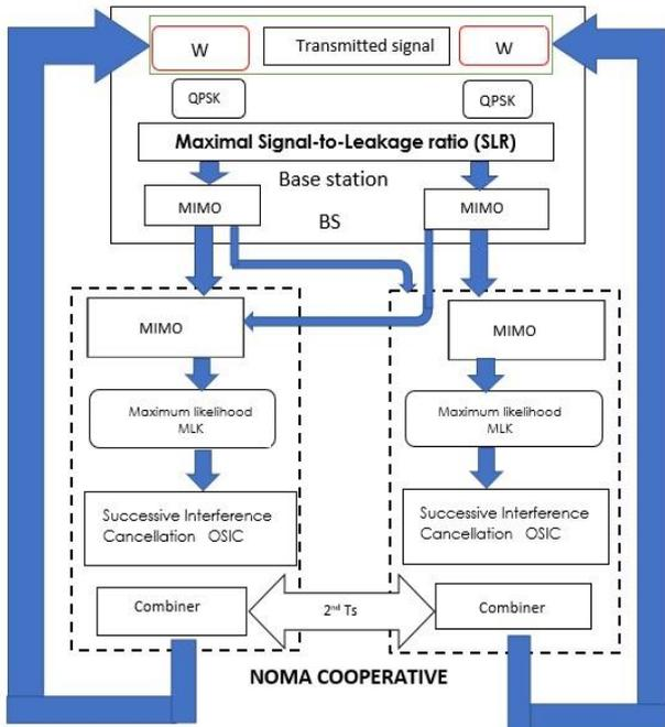
Fig. 2. Block diagram of minimizing the total transmitted power in cooperative NOMA beamforming based on maximal-SLR (MinP-NOMA-MaxSLR) proposed scheme.
