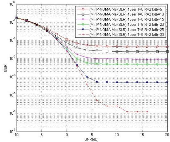
Fig. 7. BER performances (MinP-NOMA-MaxSLR) with BS  $M = 6$  antenna and 4user, each with  $N = 2$  antenna, in LOS environment of inter user channel  $SNR=20$ ,  $\beta = 0.1$
