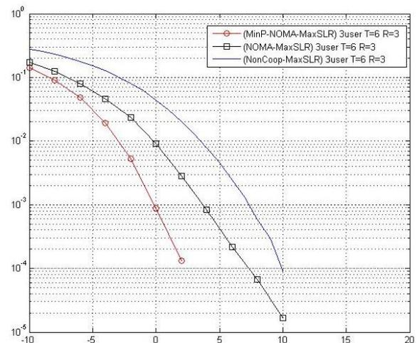
Fig. 5. BER performances of the (MinP-NOMA-MaxSLR), (NonCoop-MaxSLR) and (NOMA-MaxSLR) with BS M = 6 antenna and 3user, each with N= 3antenna, in Rician inter user channel SNR= 20 with k = 25 and  $\beta$  = 0.1.
