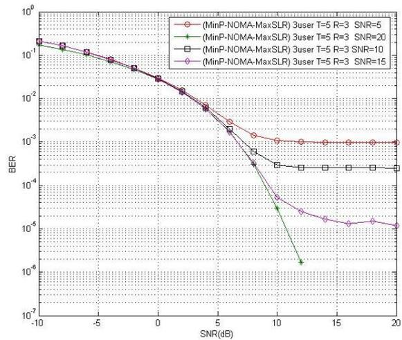
Fig. 8. BER performances of the (MinP-NOMA-MaxSLR) with BS  $M = 5$  antenna and 3 user, each with  $N = 3$ , in Rician inter user channel with  $k = 25$  and  $\beta = 0.1$ .
