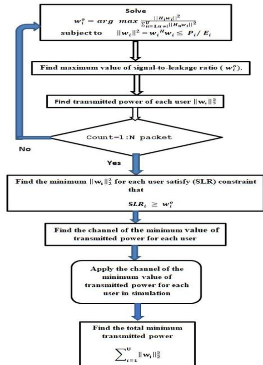
Fig. 3. Proposed Algorithm for minimizing the total transmitted power in cooperative NOMA MU-MIMO beamforming based on maximal-SLR (MinP-NOMA-MaxSLR).
