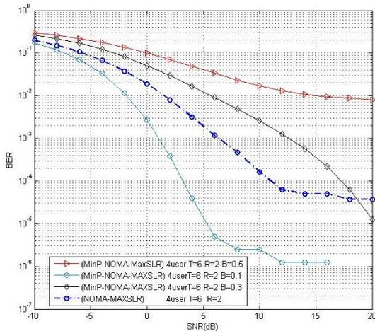
Fig. 6. BER performances of the (MinP-NOMA-MaxSLR) and (NOMA-MaxSLR) with BS  $M = 6$  antenna and 4user, each with  $N = 2$  antenna in Rician inter user channel with  $k=25$  and  $SNR= 20$ .
