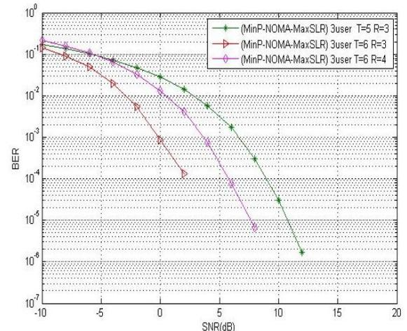
Fig. 9. BER performances of the (MinP-NOMA-MaxSLR) with BS  $M = 5$  and 6 antenna and 3user, each with  $N = 3$  and 4 antenna in Rician inter user channel  $SNR=20$ ,  $k = 25$  and  $\beta = 0.1$ .
