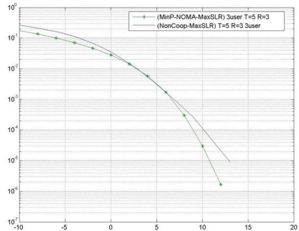
Fig. 4. BER performances of the (MinP-NOMA-MaxSLR) and (NonCoop-MaxSLR) with BS M = 5 antenna and 3user, each with N= 3, in Rician inter user channel SNR= 20 with k = 25 and  $\beta$  = 0.1.
