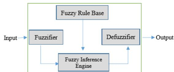
Fig. 1. The structure of fuzzy logic system
