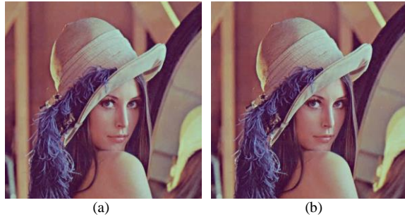
Fig. 11. Lena obtained at 0.70bpp: (a) DCT-JPEG, CPSNR=33.01dB, and (b) Improved APIDCBT-JPEG, CPSNR=33.27dB.
