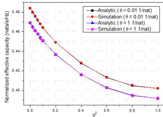
Fig. 5. Normalized effective capacity vs.  $\sigma^2$  for various QoS exponent  $\theta$ ,  $Q_{av} = 0$ (dBW),  $P_{out} = 0.1$ .
