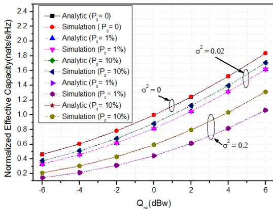
Fig. 7. Normalized effective capacity lower bounds vs.  $Q_{pk}$  for various channel estimation error  $\sigma^2$  under different values of interference-outage,  $\theta = 0.01$  (1/nat).
