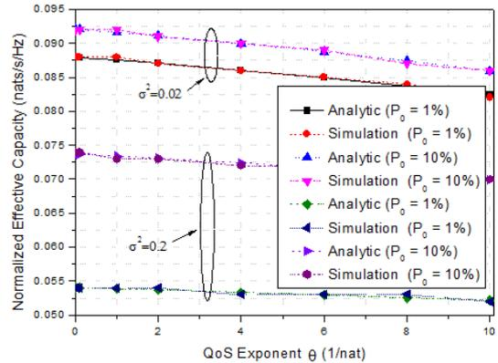
Fig. 13. Normalized effective capacity lower bounds vs. QoS exponent  $\theta$  under different value of interference-ouage,  $P_{out} = 0.1$ ,  $Q_{pk} = 0$ (dBW).
