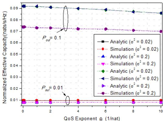
Fig. 12. Normalized effective capacity lower bounds vs. QoS exponent  $\theta$  under different outage probability,  $P_0 = 10\%$ ,  $Q_{pk} = 0$ (dBW).
