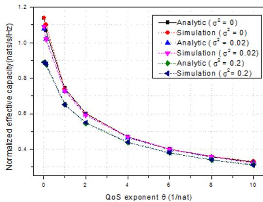
Fig. 3. Normalized effective capacity vs. QoS exponent  $\theta$  for various channel estimation error  $\sigma^2$ ,  $Q_{av} = 0$ (dBW).
