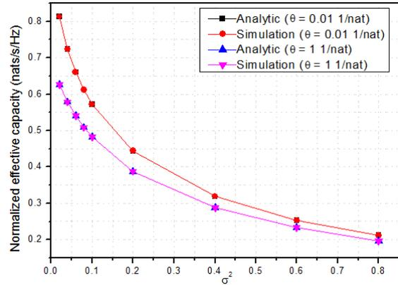
Fig. 8. Normalized effective capacity lower bounds vs.  $\sigma^2$  for various QoS exponent  $\theta$ ,  $Q_{pk} = 0$ (dBW),  $P_0 = 1\%$ .
