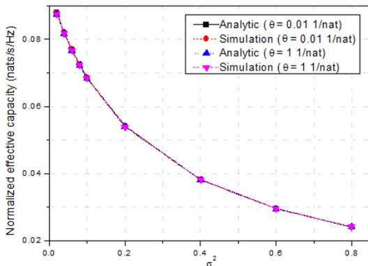
Fig. 11. Normalized effective capacity lower bounds vs.  $\sigma^2$  for various QoS exponent  $\theta$ ,  $Q_{pk} = 0$ (dBW),  $P_0 = 1\%$ ,  $P_{out} = 0.1$ .
