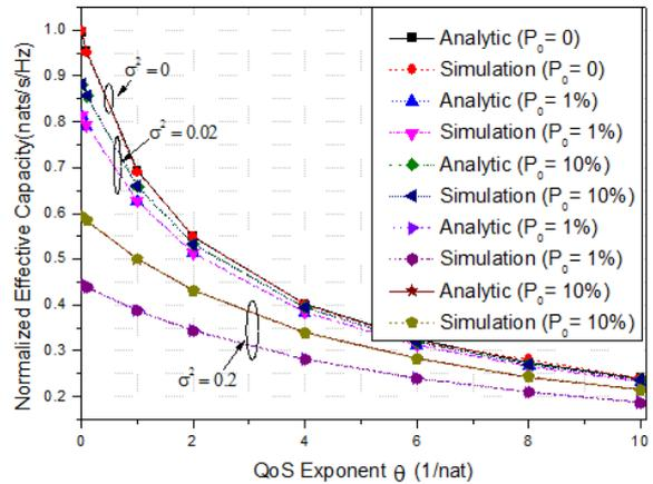
Fig. 9. Normalized effective capacity lower bounds vs. QoS exponent  $\theta$  for various channel estimation error  $\sigma^2$  under different values of interference-outage,  $Q_{pk} = 0$  (dBW).
