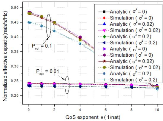
Fig. 6. Normalized effective capacity vs. QoS exponent  $\theta$  for various channel estimation error  $\sigma^2$ ,  $Q_{pk} = 0$ (dBW).
