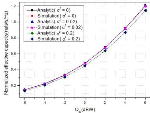
Fig. 4. Normalized effective capacity vs.  $Q_{av}$  for various channel estimation error  $\sigma^2$ ,  $\theta = 0.01$  (1/nat),  $P_{out} = 0.1$ .
