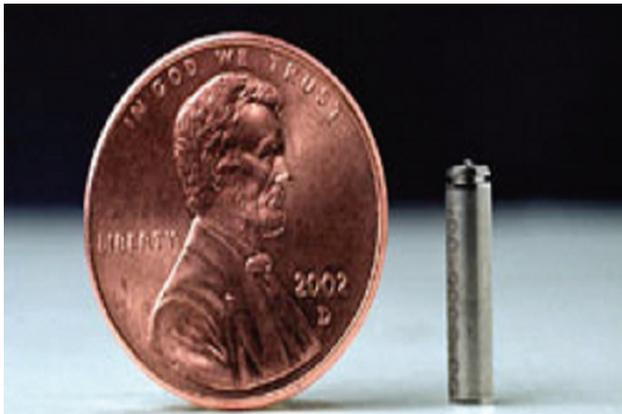
Fig. 5 Rechargeable Li Ion battery for implant devices
