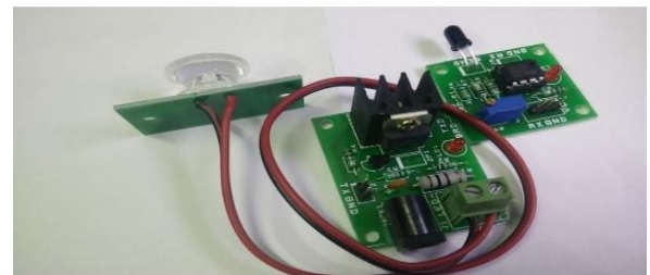
Fig. 4. LiFi Transmitter and receiver module.
