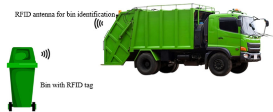
Fig. 10. RFID system for identifying and tracking waste bins.
