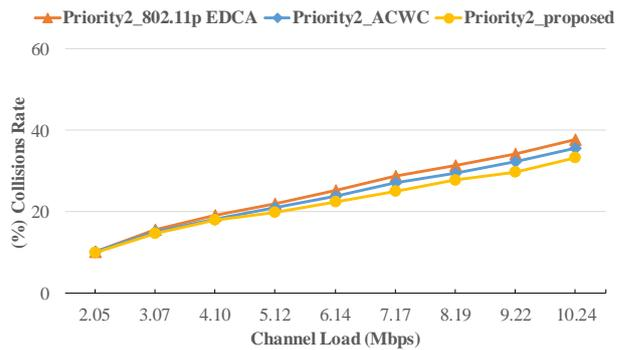
Figure 4. Priority 2 traffic collision rate in urban highway model.
