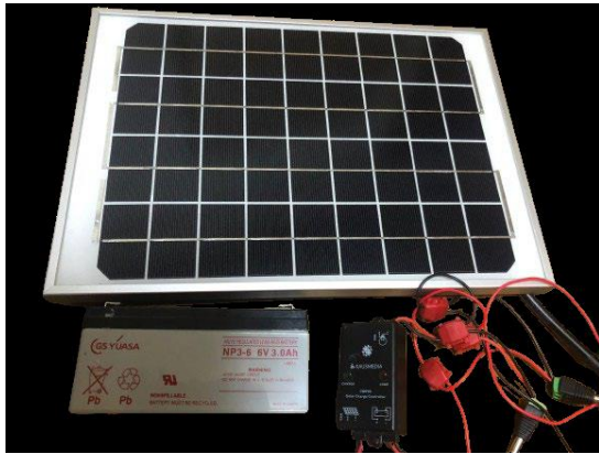
Figure 1 The developed power supply system.
