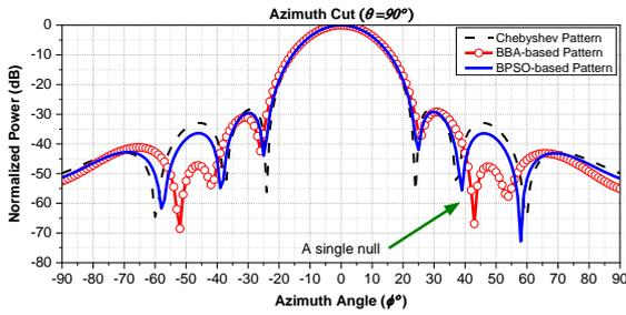
Figure 8. The 2D optimized patterns with a single null.
