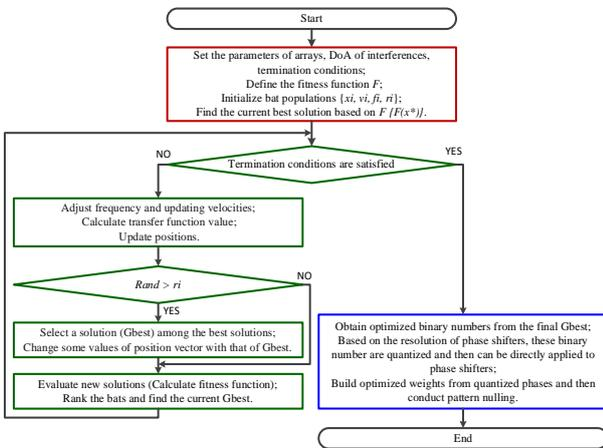
Figure 2. The flowchart of the proposed algorithm.
