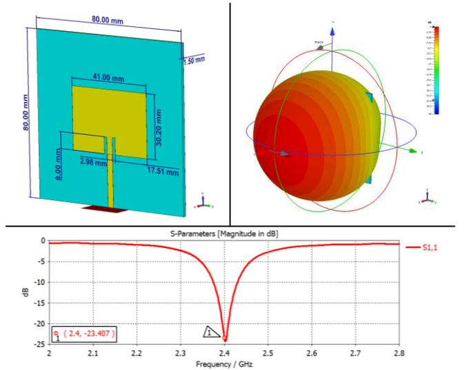
Figure 3. The characteristics of a patch antenna designed in CST.
