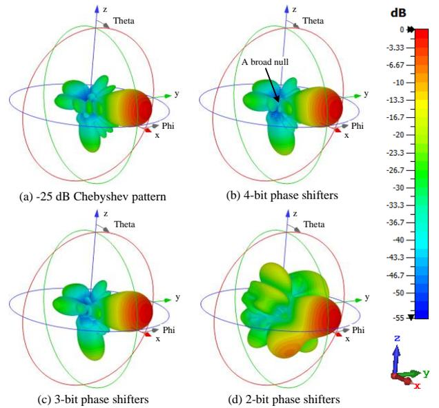
Figure 12. The 3D patterns with the different resolutions of phase shifters.
