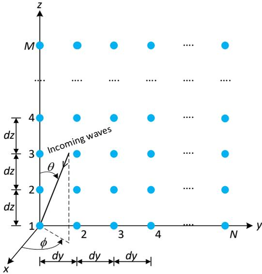
Figure 1. A URA with  $M \times N$  elements.
