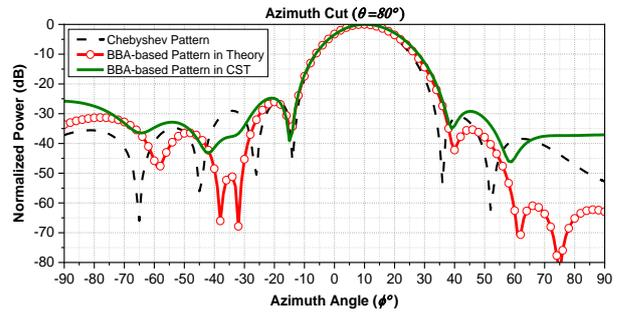
Figure 11. The 2D patterns when using 4-bit phase shifters.
