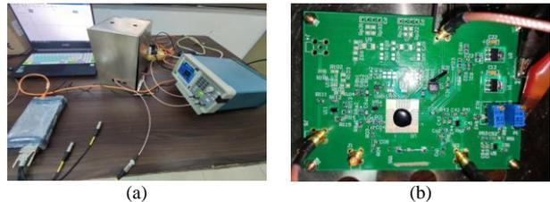
Fig. 16. The test system. (a) The overall test system; (b)The analog amplifier circuit board.
