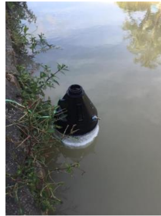
Fig. 18. Sensor buoy for dissolved oxygen measurements
