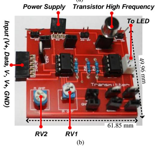
Fig. 8. Hardware prototype of proposed Bias-T
