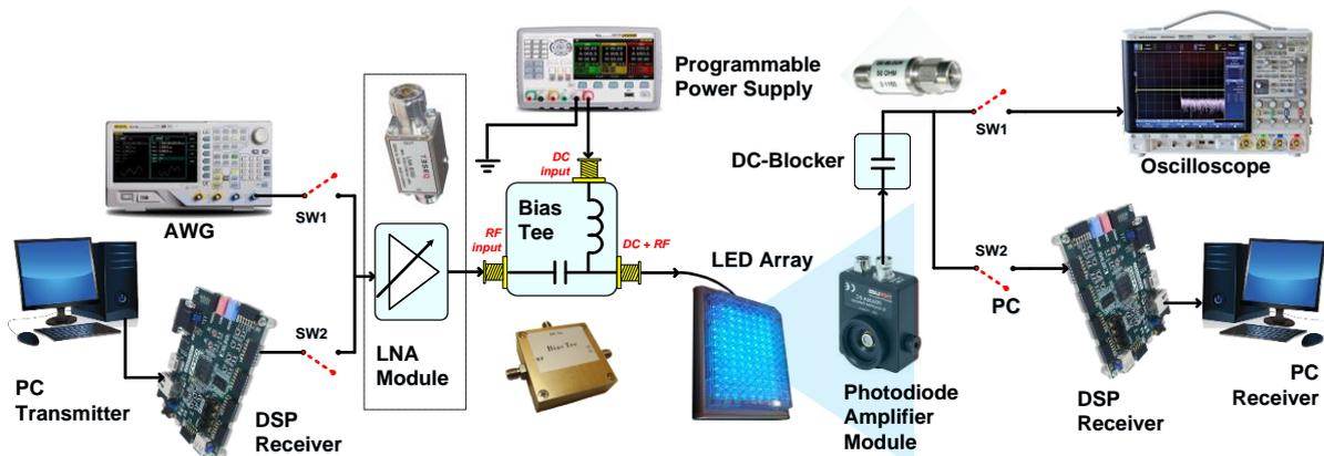
Fig. 1. Generic architecture of the high-speed VLC system utilizing commercial modules
