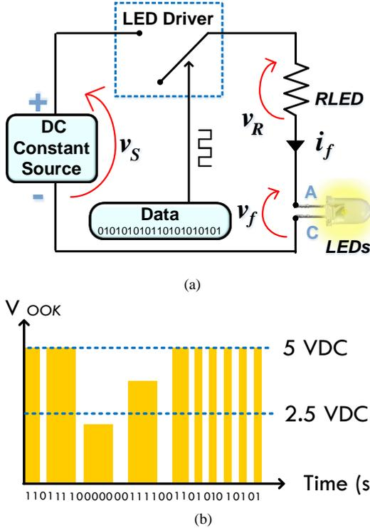
Fig. 2. Switch LED driver: (a) the basic electronic circuitry of VLC system that uses digital modulation with constant amplitude, in this case is OOK signal. This illustration is reproduced from [25]; (b) brightness control on the LED light uses ARDUINO board as DSP module when 5 V<sub>DC</sub> as reference voltage for logic high in which an amplitude above 2.5 V<sub>DC</sub> is considered as logic “1” and under 2.5 V<sub>DC</sub> is considered as logic “0”, reproduced from [26]
