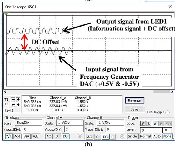
Fig. 7. LED driver simulation: (a) circuit simulation; (b) signal capture on a virtual oscilloscope on MULTISIM V.14 comparing the input signal with the LED anode (Simulation settings are single carrier signal = sinusoid, amplitude = 0.5 Vpp, input frequency = 500 kHz)
