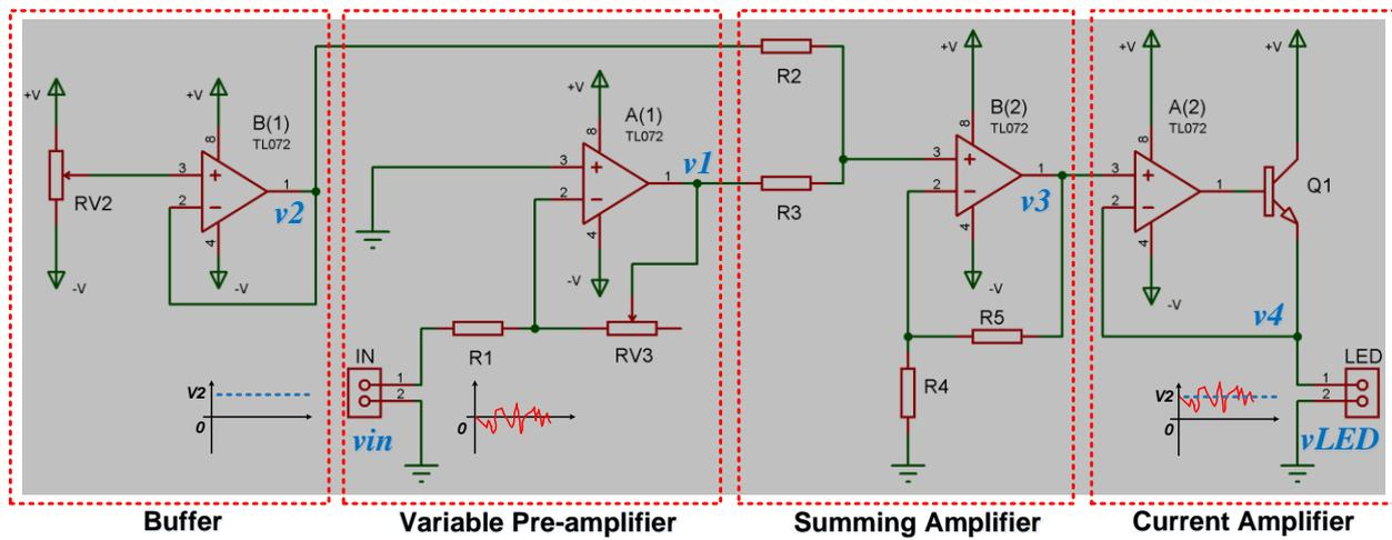
Fig. 3. The proposed Bias-T network/Linear LED driver circuitry
