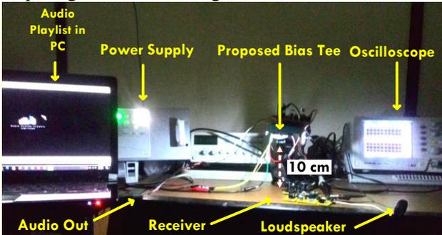
Fig. 9. A photograph of performance test of the proposed Bias-T for 3<sup>rd</sup> scenario. The room condition is 0 lux.
