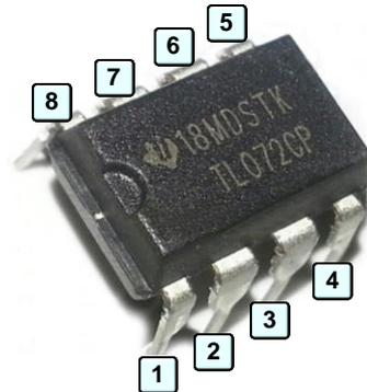
Fig. 5. A photograph of physical form of TL072 that has four pins (1 = Output A, 2 = Inverting A, 3 = Non-inverting A, 4 =  $V_{EE}$ , 5 = Non-inverting B, 6 = Inverting B, 7 = Output, and 8 =  $V_{CC}$ )
