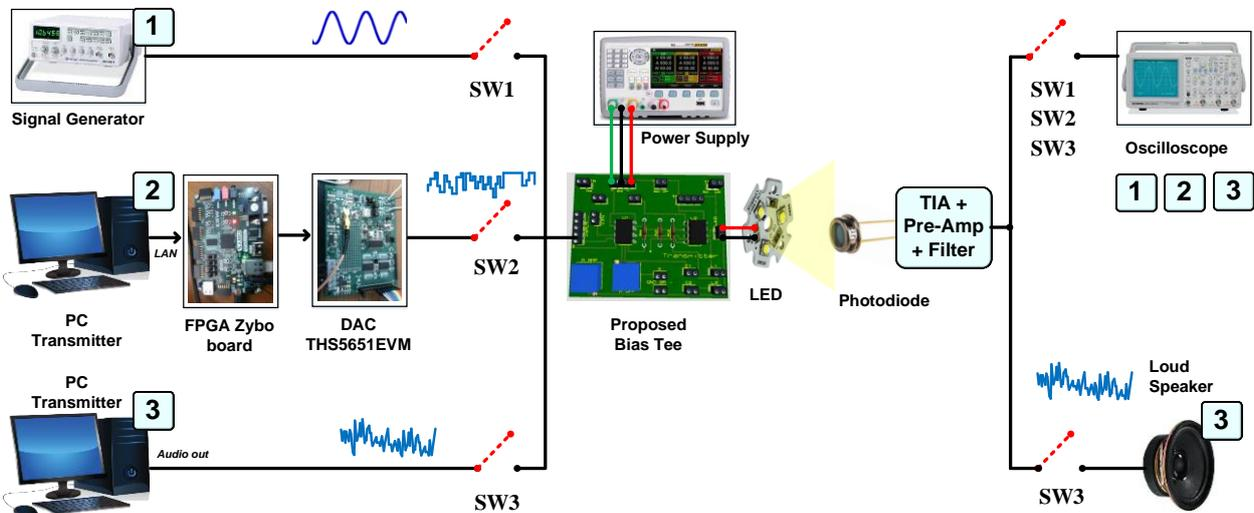
Fig. 6. POC of the proposed Bias-T, the switch SW1, SW2, and SW3 for choosing the test configuration
