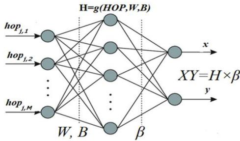
Fig. 3. The based hops single ELM localization model
