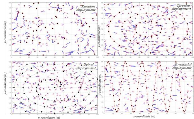
Fig. 5. Samples of localization results for Random, Circular, Spiral and Sinusoidal anchors deployment scenarios
