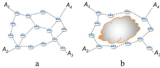
Fig. 1. (a) Isotropic WSN deployment (without obstacles), (b) Anisotropic WSN deployment (with obstacles)
