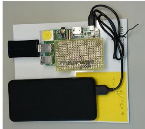
Fig. 1. Mesh node developed by us.
