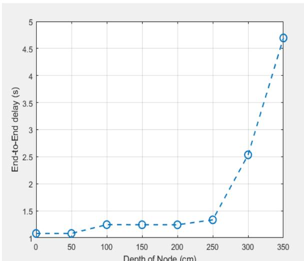
Fig. 3. End to end delay vs depth (Experiment 1).
