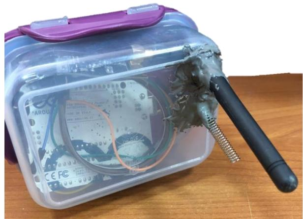
Fig. 1. Hardware setup of the node.
