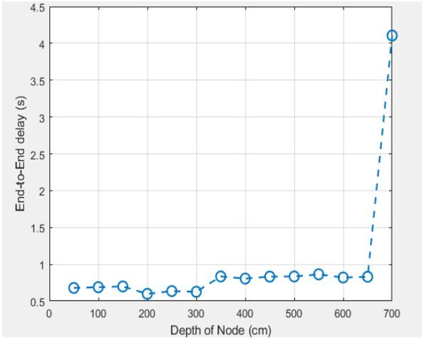
Fig. 6. End to end delay vs depth (Experiment 2).
