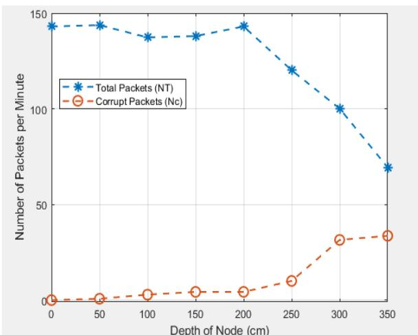
Fig. 4. Packets count over depth (Experiment 1)
