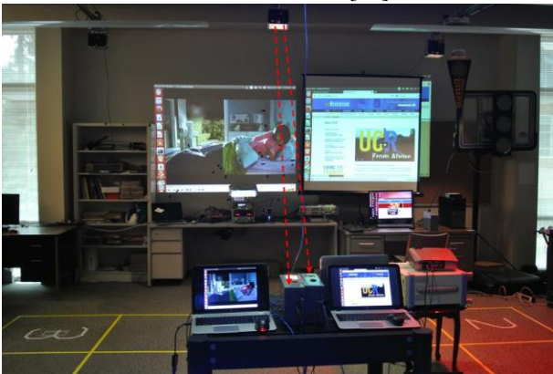
Fig. 7. A two-user LED VLC system for high-definition video streaming over light [14].
