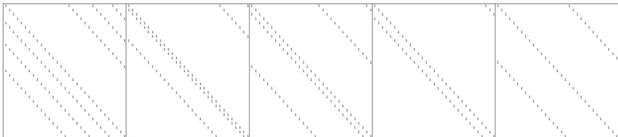
Figure 1. Parity-check matrix of the proposed QC LDPC code with  $n=155$  and  $R=4/5$ .
