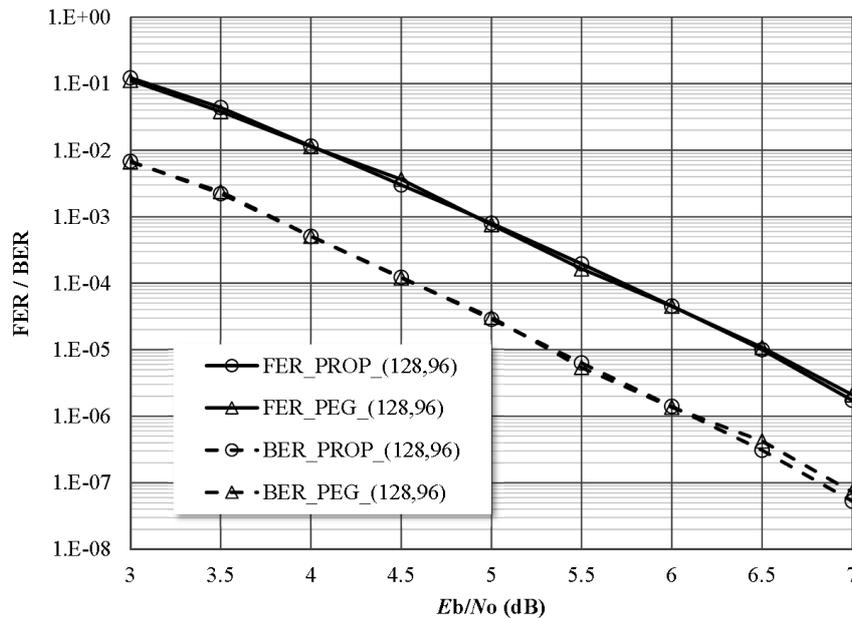
Figure 4. FER and BER of the proposed QC LDPC code and the PEG LDPC code for  $n=200$  and  $R=4/5$ .
