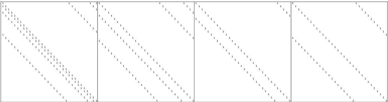
Figure 2. Parity-check matrix of the proposed QC LDPC code with  $n=128$  and  $R=3/4$ .
