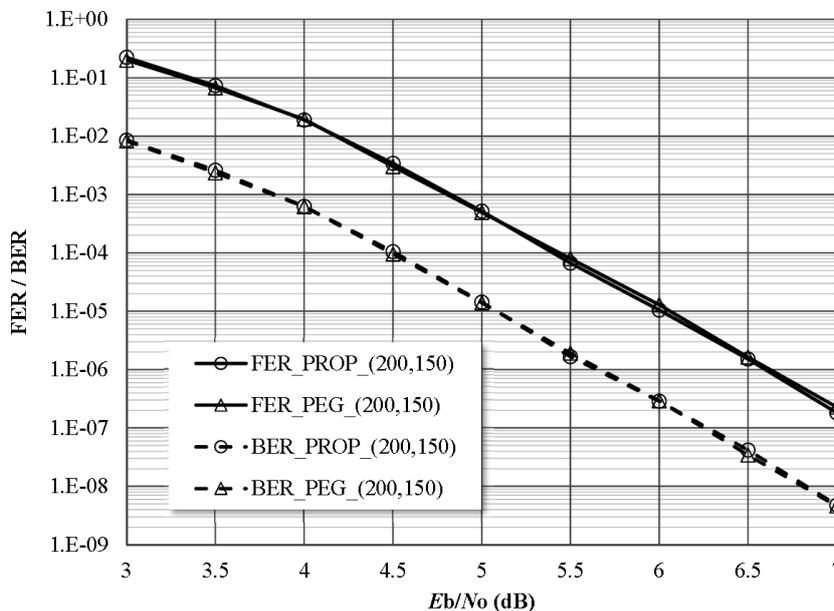
Figure 3. FER and BER of the proposed QC LDPC code and the PEG LDPC code for  $n=200$  and  $R=4/5$ .
