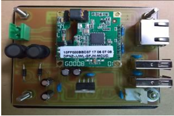
Fig. 9. The implemented DC-based PLC transceiver module.
