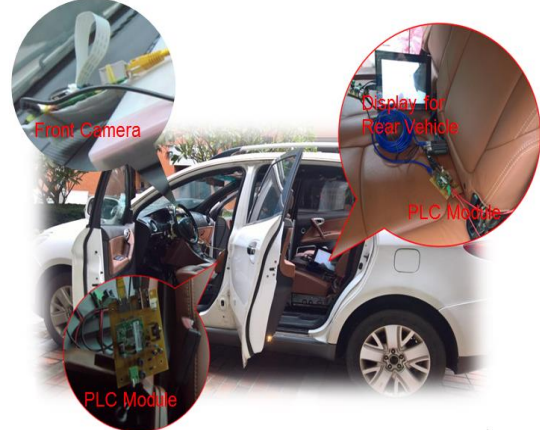
Fig. 11. The DC-based PLC transceiver tested on a real vehicle.
