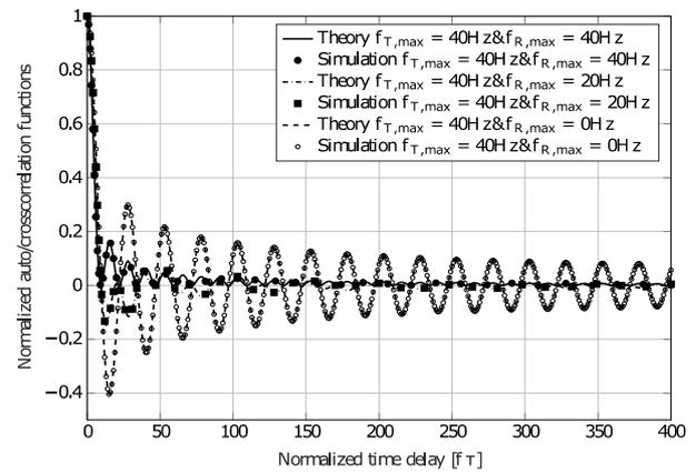
Fig. 2. Theoretical and simulated autocorrelation / cross-correlation functions of  $2e^6$  generated Rayleigh fading samples
