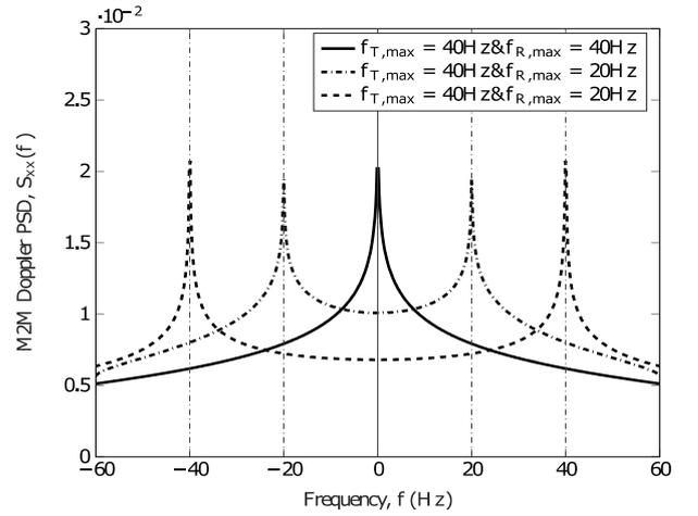
Fig. 1. The M2M double-Doppler PSD for various combinations of the maximum Doppler frequencies  $f_{T,\max}$  and  $f_{R,\max}$ .
