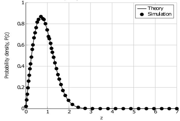
Fig. 1. The PDF  $P_R(r)$  of the envelope of the double Rayleigh process  $\mu(t)$
