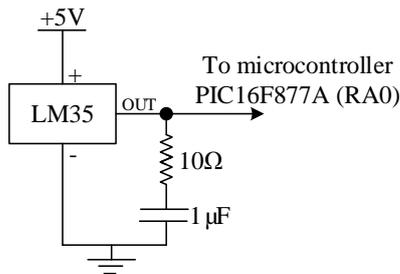
Fig. 2. Schematic of temperature sensor LM35.
