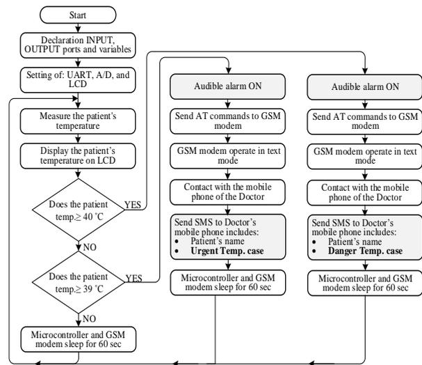
Fig. 4. Flow chart of the temperature measurements of patients and proposed sleep/wake algorithm.
