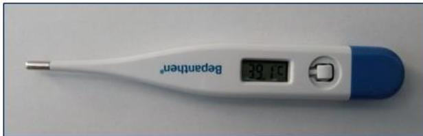
Fig. 9. Benchmark (digital thermometer) adopted in the experiment.
