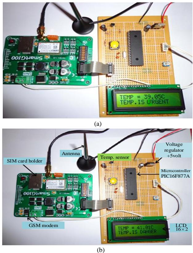
Fig. 7. RTRMS at (a) urgent case and (b) danger case.
