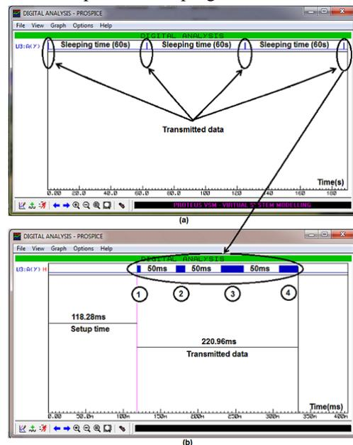
Fig. 5. Digital analysis of (a) transmitted data with sleep time and (b) transmitted data for one packet.
