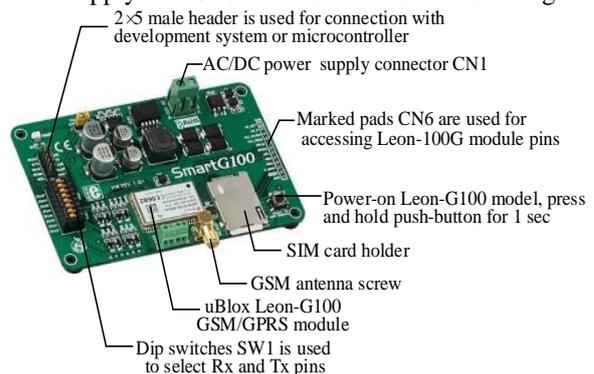
Fig. 3. SmartG100 with uBlox Leon-G100 module.
