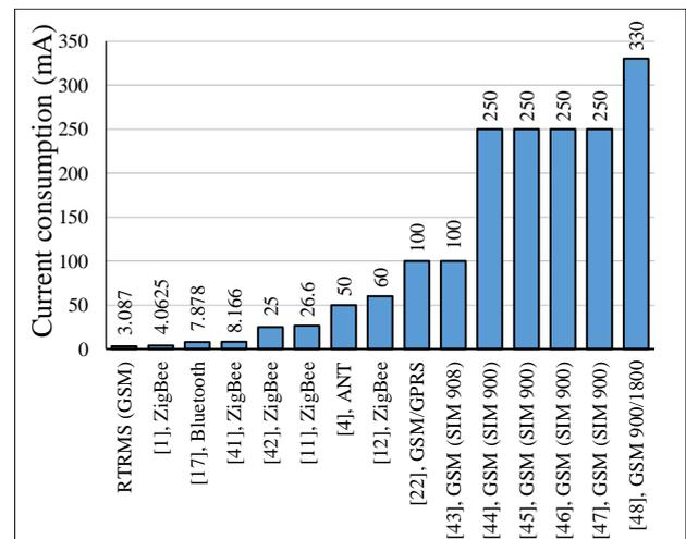
Fig. 12. Bar chart comparing current consumption requirements for existing works with proposed RTRMS.
