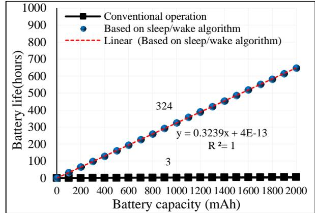
Fig. 11. Expected battery life versus practical battery capability in the RTRMS.
