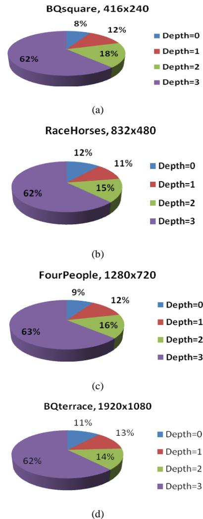
Fig. 3. Time-consumption distribution of different CU depths.
