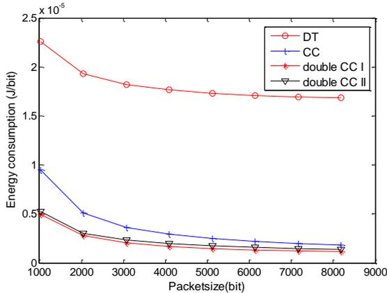
Fig. 6. Energy consumptions under different data packet sizes
