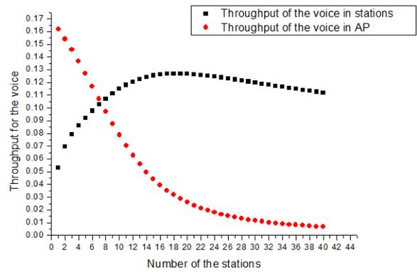
Fig. 8. Throughput of the voice traffic in stations and AP.
