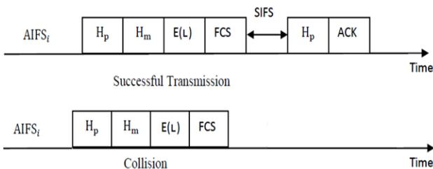
Fig. 7. Basic access method frames.
