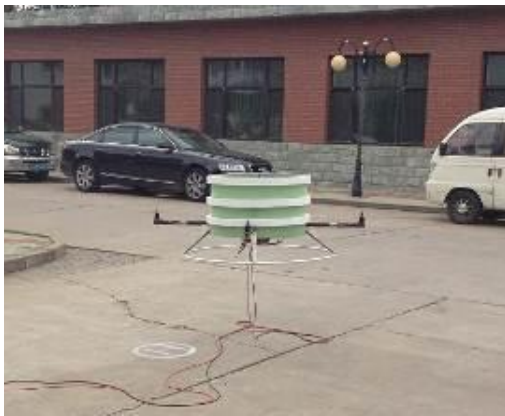
Fig. 4. A tethered multi-rotor UAV. The black and red wires on the ground are the power supplying cable.
