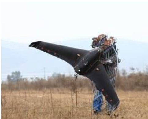
Fig. 2. Fixed wing UAV for power inspection
