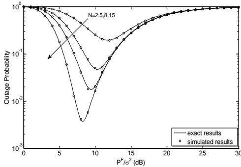
Fig. 6. Outage probability versus SNR  $P^F/\sigma^2$  for FTP.
