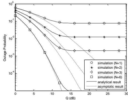
Fig. 5. Outage probability versus tolerable interference power for ATP ( $Q_1 = Q_2 = Q$ ).
