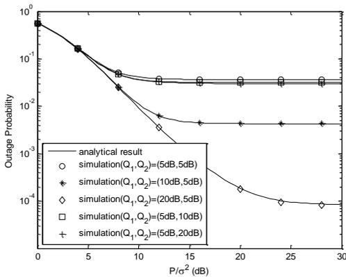
Fig. 4. Outage probability versus SNR  $P/\sigma^2$  for ATP.
