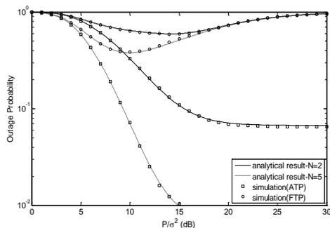
Fig. 7. Outage probability comparison of FTP and ATP.
