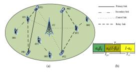
Fig. 1. Cooperative cognitive radio networks (a) system architecture (b) time duration division.
