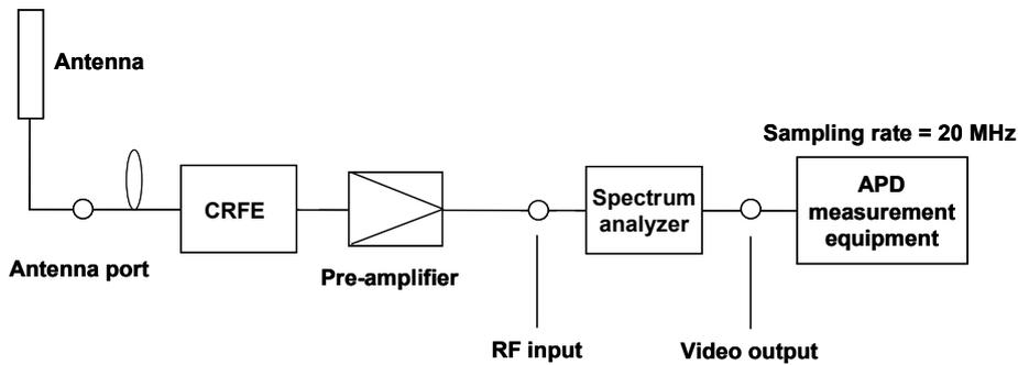
Figure 7. Configuration of APD measurement experiment.
