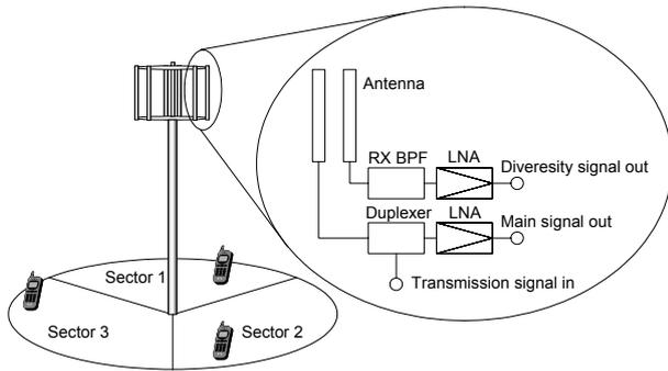
Figure 1. Basic configuration of a three-sector cellular base station.
