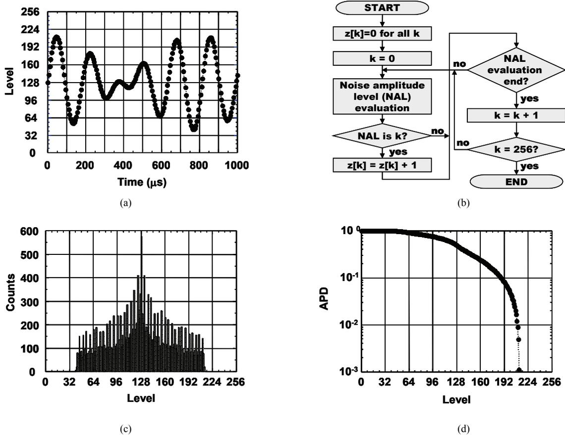
Figure 8. Statistical process using APD measurement equipment. (a) Sampled noise waveform. (b) Noise amplitude level (NAL) evaluation. (c) Histogram. (d) APD.
