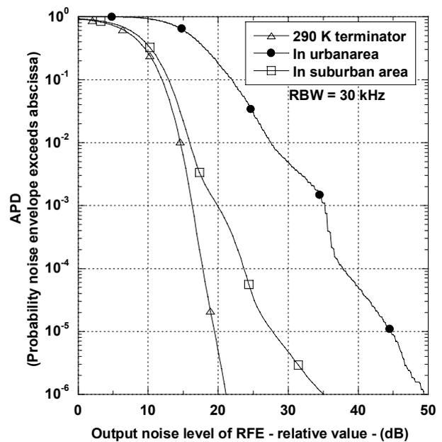
Figure 12. APD of antenna noise measured in VHF band.
