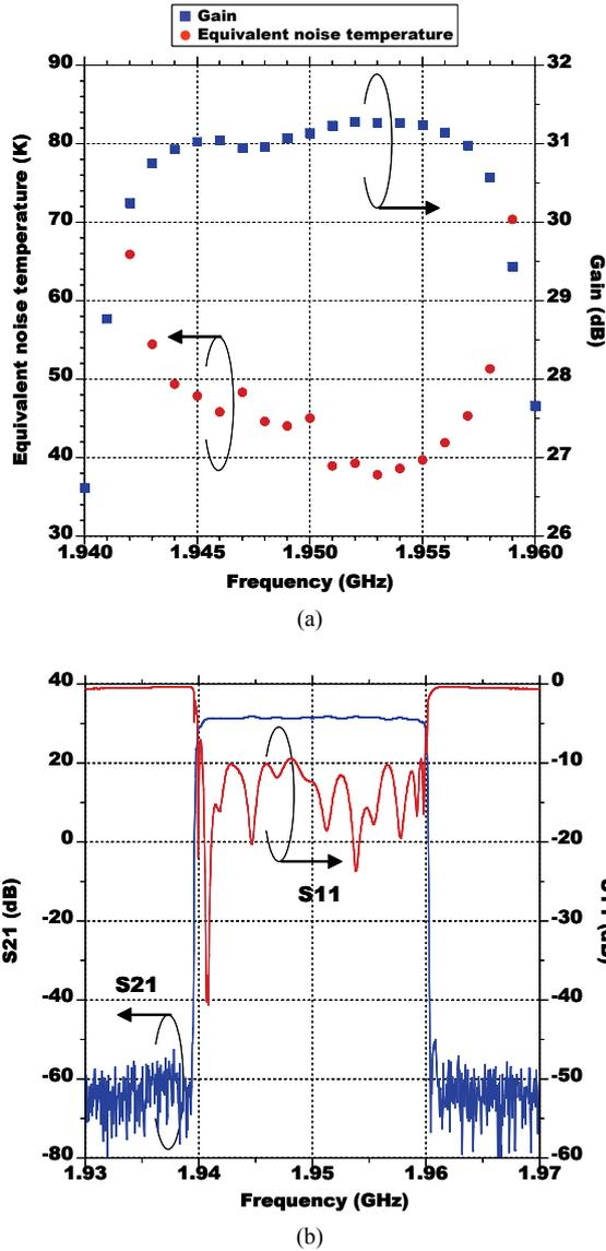
Figure 4. RF performance example of experimental CRFE measured at 70 K. (a) Equivalent noise temperature and gain. (b) Frequency characteristics.
