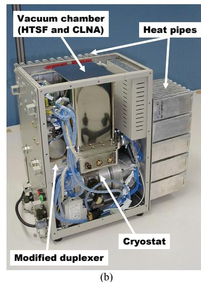
Figure 3. Experimental CRFE. (a) Basic configuration. (b) Photograph.
