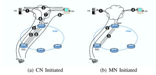
Fig. 2. Signaling prior to data transmission (a) CN initiated communication, (b) MN initiated communication.
