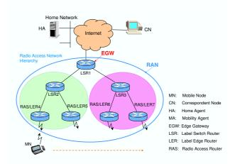
Fig. 1. Mobile MPLS Radio Access Network
