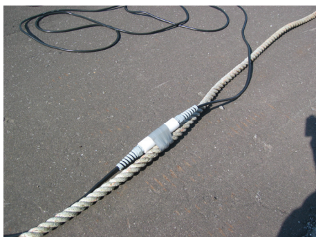
Figure 8. Thermometer and cable set up in mooring rope.
