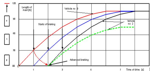
Fig.2. An illustration of the impact of i-radar system: the vehicle 2 receives a warning signal from vehicle 0 at  $t=1s$  and starts to brake at  $t=2s$  along the dotted trajectory and avoids a collision
