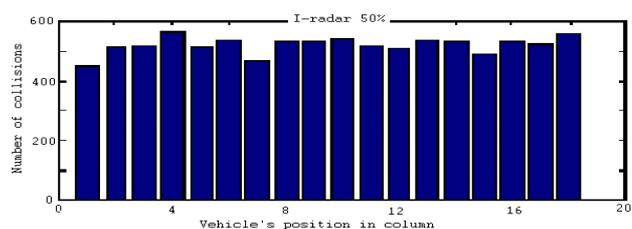
Fig.5d. Distribution of light collisions down the position in column. Penetration of i-radar 50%
