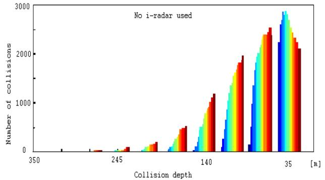
Fig.5a. Distribution of collisions down their depth and vehicle's position in column. No i-radar used. Number of scenarios 10000
