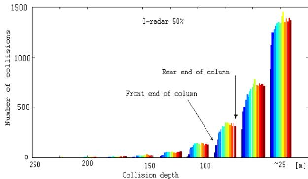
Fig.5b. Distribution of collisions down their depth and vehicle's position in column. I-radar penetration 50%. Number of scenarios 10000
