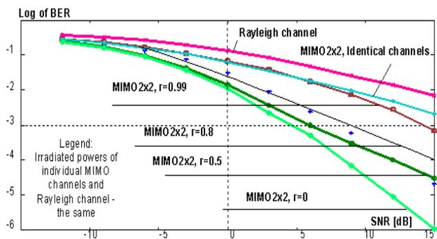
Fig.8. BER vs. SNR for MIMO2x2 system with- and without channel cross-correlation
