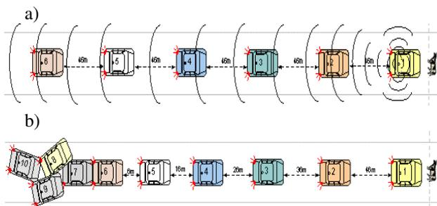
Fig.1. Deployment of vehicles after an abrupt stop of the leader (1) for the case of i-radar used (a) and not used (b)
