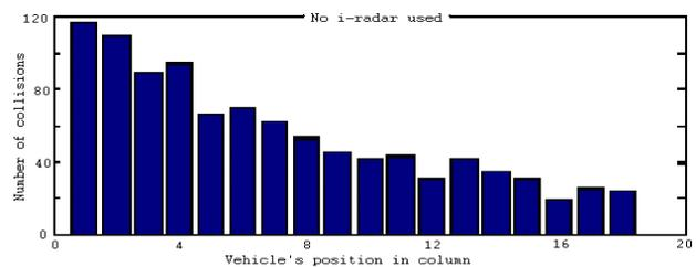
Fig.5c. Distribution of light collisions for the case of no i-radar used
