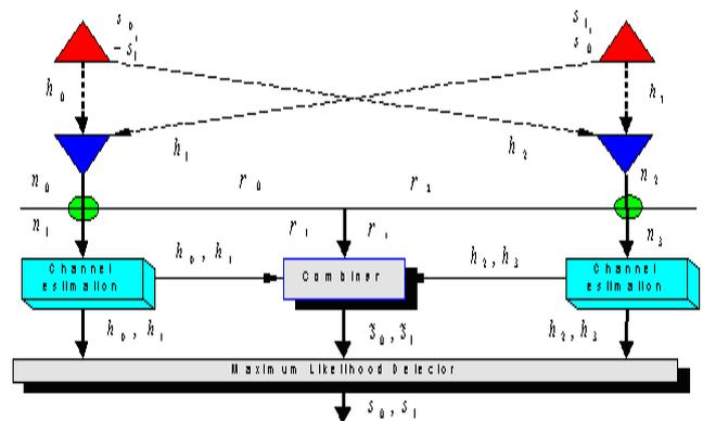
Fig.7. Main factors of the reception process in MIMO2x2 system
