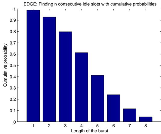
Figure 9. Cumulative probability of finding bursts with a blocking probability of 1%
