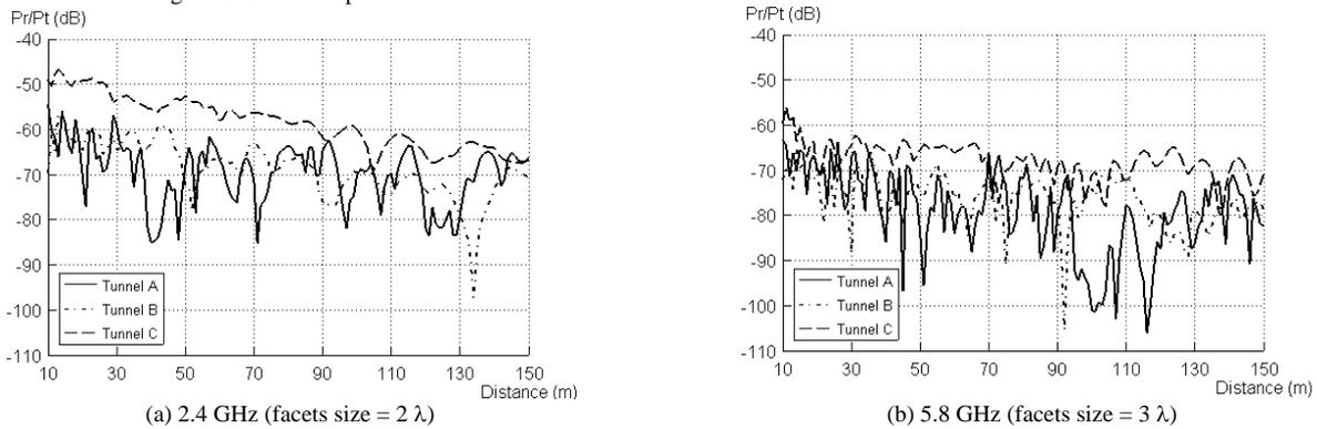
Figure 7: Simulated path loss as a function of the distance - Tunnels A, B, C
