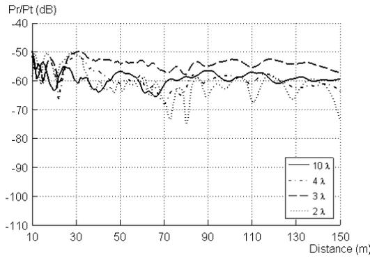
Figure 2: Simulated path loss as a function of the distance for different sizes of the tunnel facets - Tunnel C - 1 GHz
