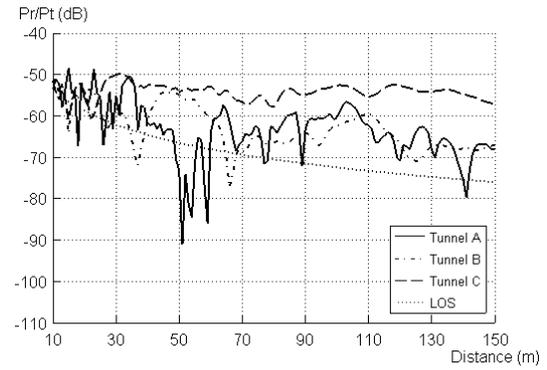
Figure 3: Simulated path loss as a function of the distance - Tunnels A, B, C (facets size = 3λ) - 1 GHz
