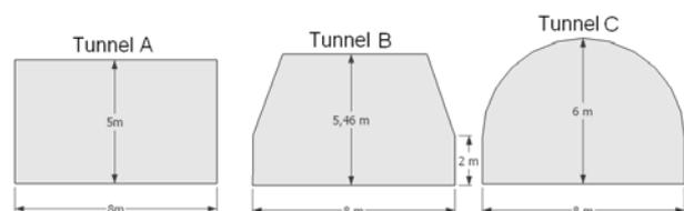
Figure 1: Geometry of tunnels
