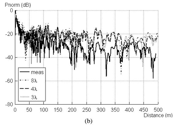
Figure 11: Simulated and measured path loss as a function of the distance for different sizes of the tunnel facets - 5.8 GHz
