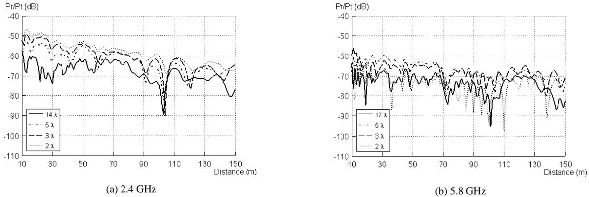
Figure 6: Simulated path loss as a function of the distance for different sizes of the tunnel facets - Tunnel C
