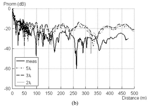
Figure 10: Simulated and measured path loss as a function of the distance for different sizes of the tunnel facets - 2.4 GHz
