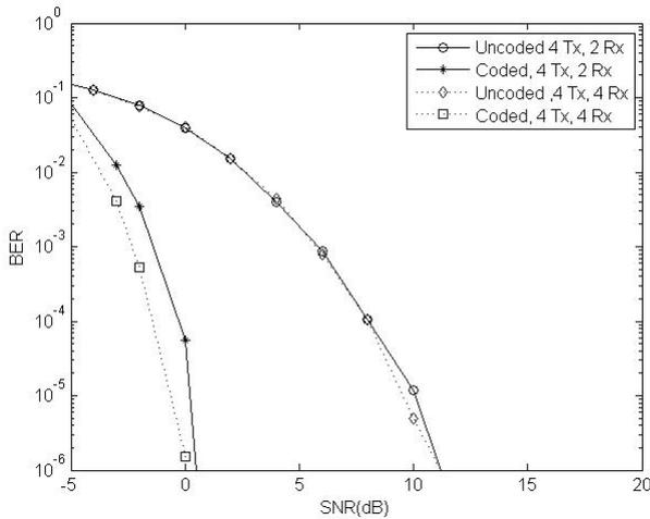
Fig. 10 BER performance comparison of coded MIMO-OFDM system (4Tx & 2/4 Rx) and uncoded MIMO-OFDM system with same diversity
