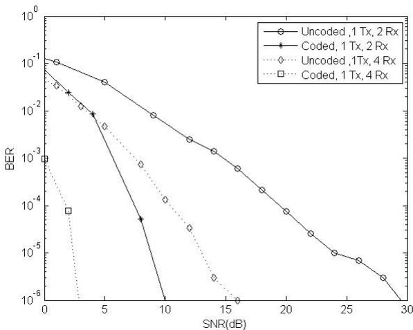
Fig. 7 BER performance comparison of coded SIMO-OFDM and uncoded SIMO-OFDM system
