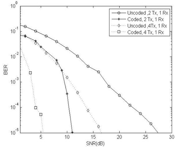
Fig. 8 BER performance comparison of coded MISO-OFDM and uncoded MISO-OFDM system
