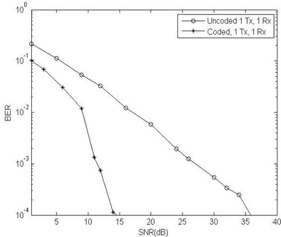
Fig. 6 BER performance comparison of coded SISO-OFDM and uncoded SISO-OFDM system
