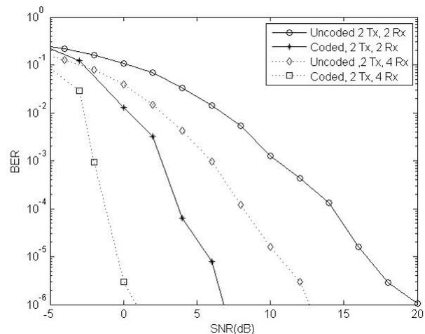
Fig. 9 BER performance comparison of coded MIMO-OFDM system (2 $T_x$  & 2/4  $R_x$  ) and uncoded MIMO-OFDM system with same diversity.
