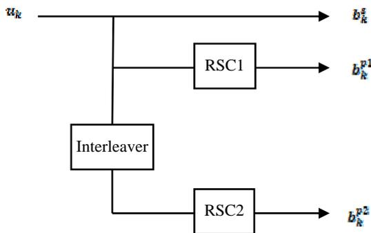
Fig. 3. Structure of Turbo Encoder
