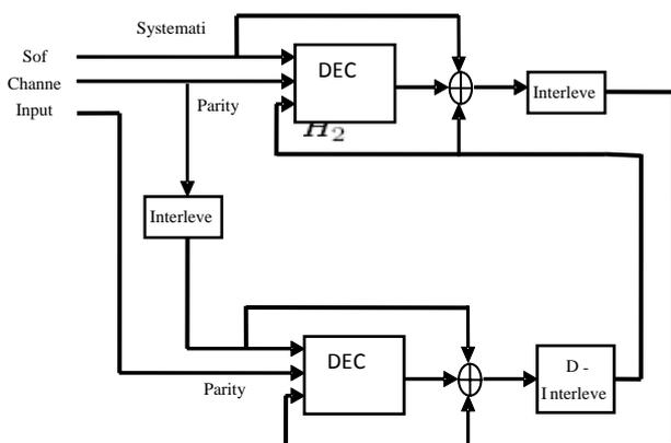
Fig. 5. Block diagram of turbo decoder
