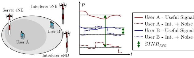
Figure 2. Main issues associated to interference control.
