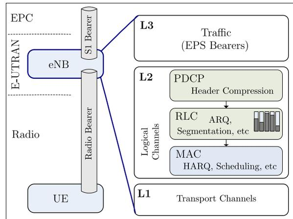
Figure 3. LTE structure/protocols for downlink traffic.
