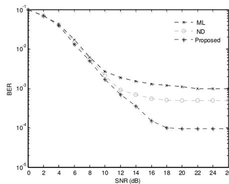
Figure 12. Comparison of BER versus SNR (dB) curves for a synchronous BPSK/DS CDMA system in a Gaussian channel for a large value of  $K$ .
