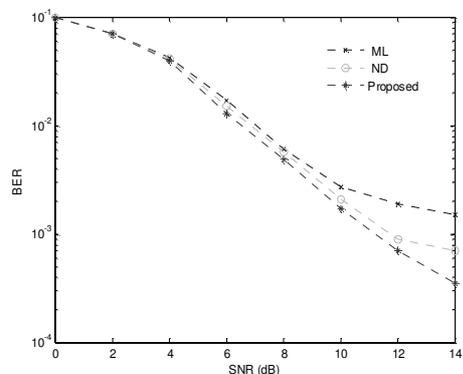
Figure 11. Comparison of BER versus SNR (dB) curves for a synchronous BPSK/DS CDMA system in a Gaussian channel for a large value of  $K$ .
