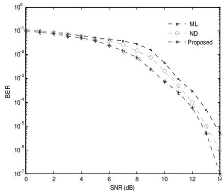
Figure 10. Comparison of BER versus SNR (dB) curves for a synchronous BPSK/DS CDMA system in a Gaussian channel for a small value of  $K$ .
