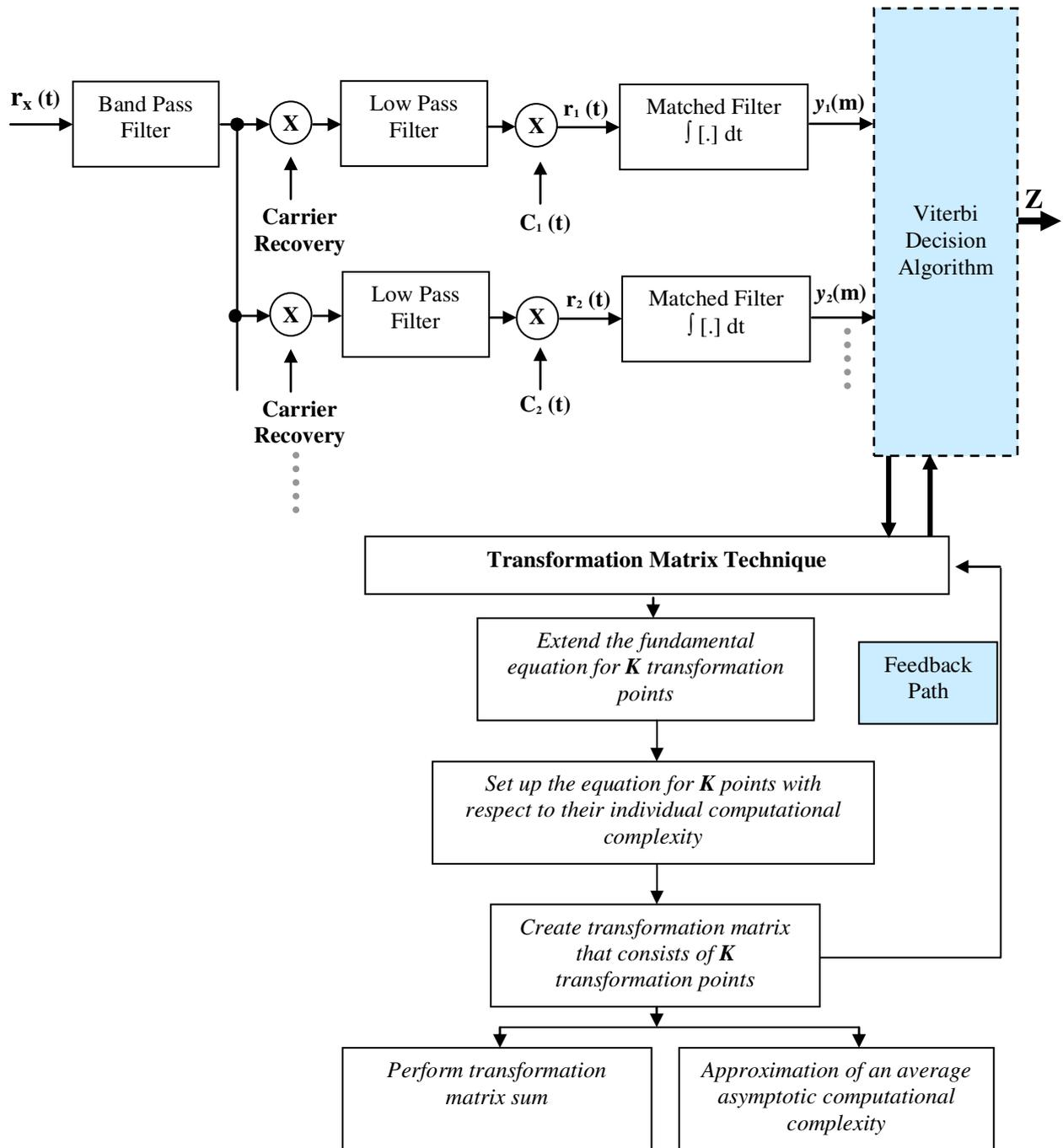
Figure 1. Implementation of proposed transformation matrix (TM) algorithm with the optimum multiuser receiver
