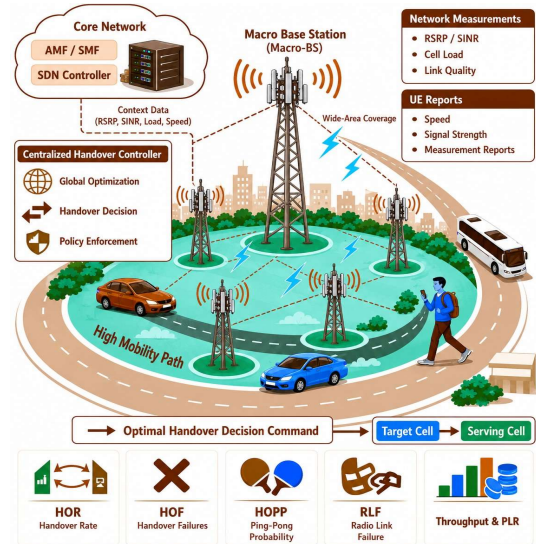
Fig. 2. Ultra-dense 5G heterogeneous network simulation architecture with centralized handover management.
