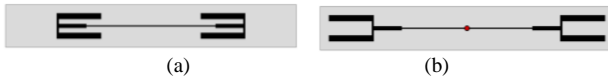
Fig. 3. Collinear dipole antenna with two layers with different sides (Mode B), (a) front view, (b) bottom view.
