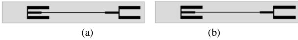
Fig. 2. Collinear dipole antenna with two layers with different sides (Mode A), (a) front view, (b) bottom view.
