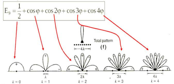
Figure 5. Antenna array with uniform spacing.
