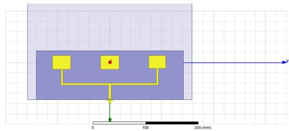
Figure 6. 1×3 antenna design without parasitic.
