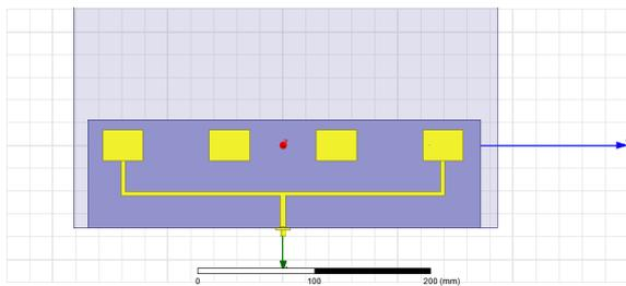
Figure 8. 1×4 antenna design with with parasitic
