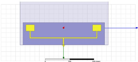
Figure 9. 1×4 antenna design with without parasitic.
