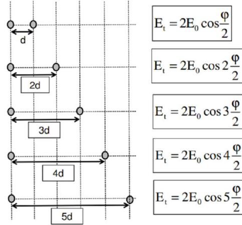
Figure 4. The field generated by an array antenna with uniform spacing.
