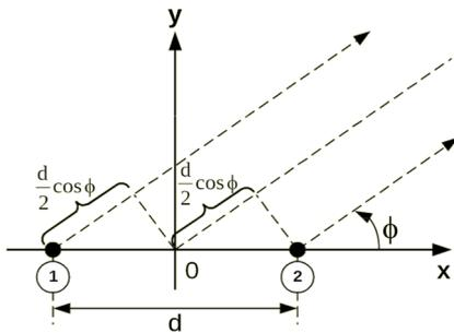
Figure 3. Antenna array with uniform spacing.
