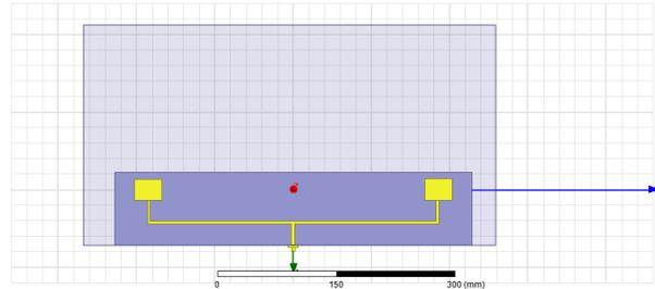
Figure 11. 1×5 antenna design without parasitic.
