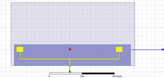
Figure 13. 1×6 antenna design with without parasitic.
