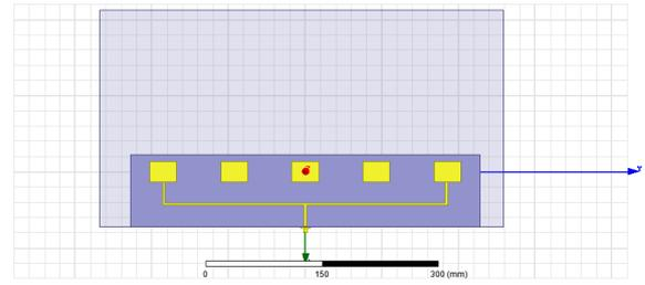
Figure 10. 1×5 antenna design with parasitic.
