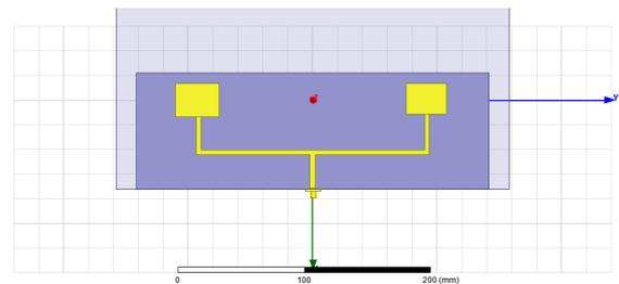
Figure 7. 1×3 antenna design with parasitic.
