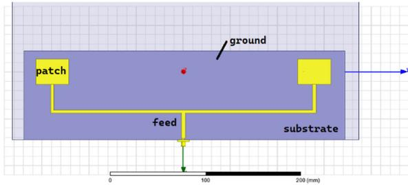
Figure 1. Conventional patch microstrip antenna.
