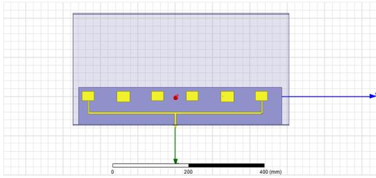
Figure 12. 1×6 antenna design with parasitic.
