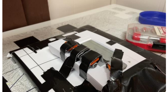
Figure 2. IoT device (Sensi-Thermostat) with physically enlarged buttons to eliminate robotic arm misalignment errors.
