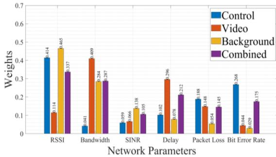
Figure 3. Fuzzy weights of network parameters for different traffic classes.
