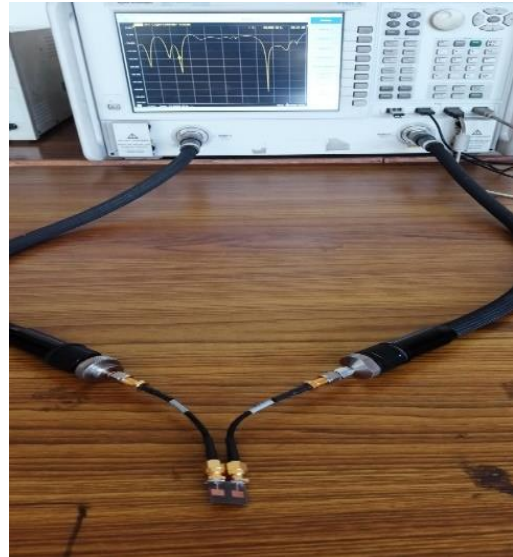
Figure 6. Experimental setup for the measurement of S-parameter of Fabricated 2-port Multiple Antenna
