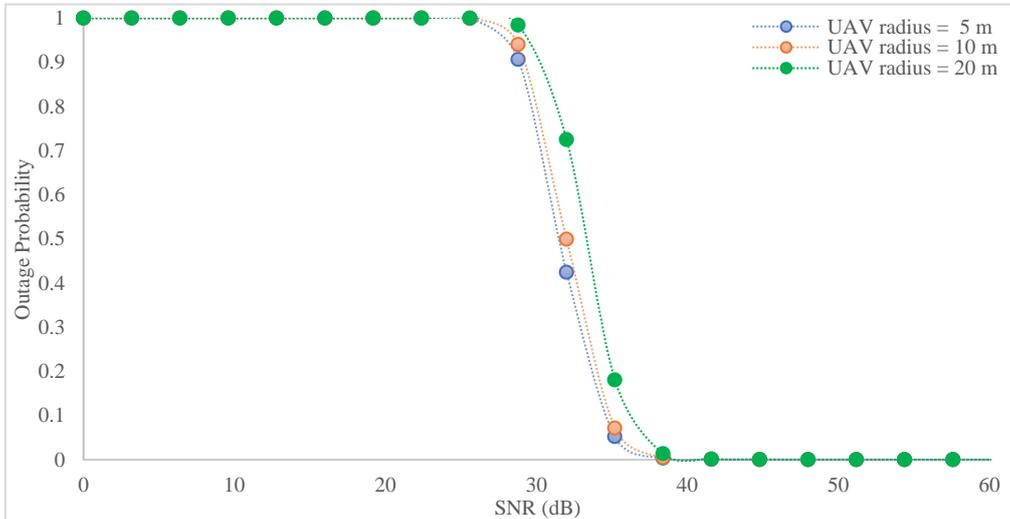
Figure 6. The output of outage probability and SNR value at different UAV radius (5 m, 10 m, 20 m).
