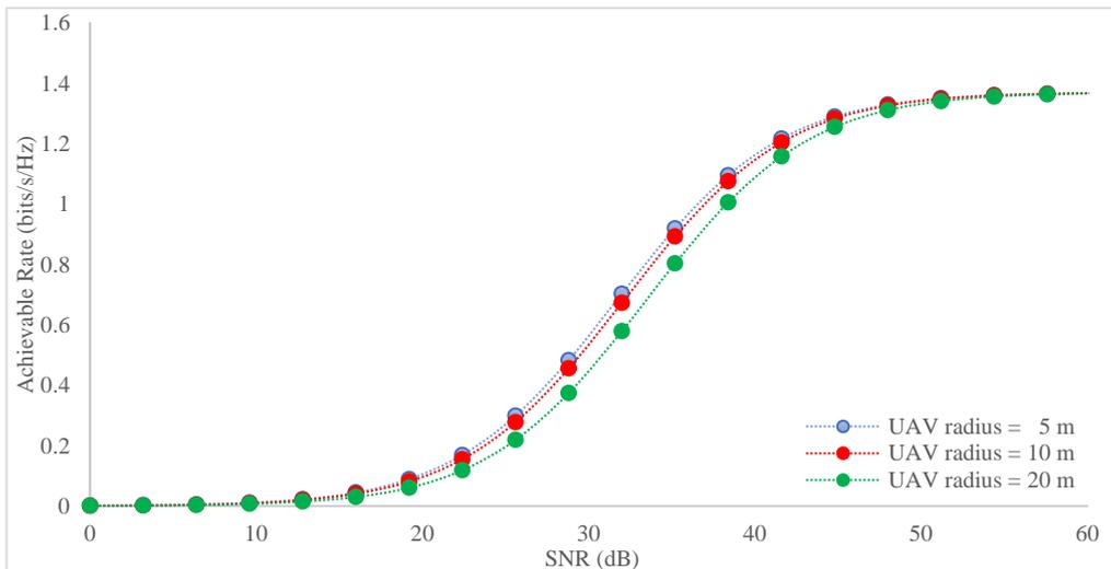
Figure 7. The output of the achievable rate and SNR value at different UAV radius (5 m, 10 m, 20 m).
