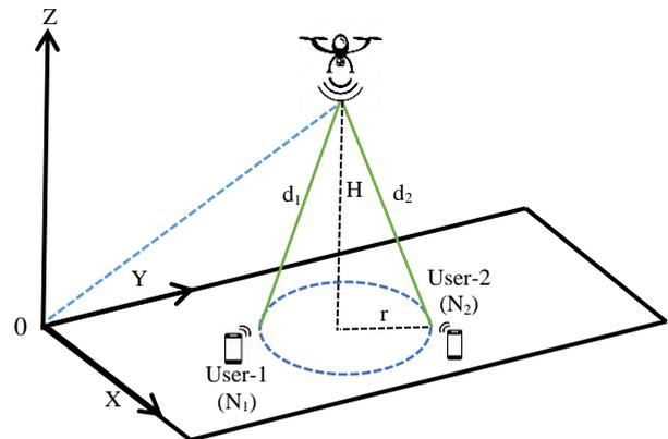
Figure 3. Illustration of UAV- BS in a disaster-affected area.
