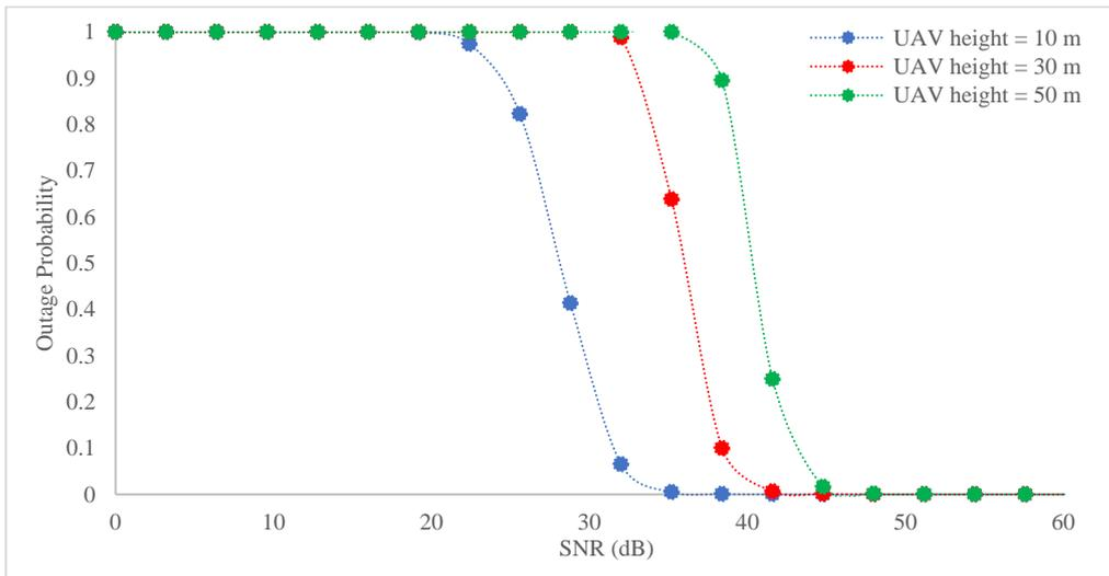
Figure 4. The output of outage probability and SNR value at different UAV altitudes (10 m, 30 m, 50 m).
