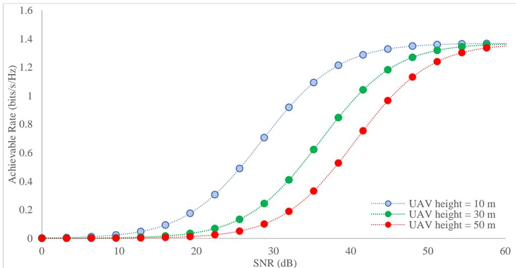
Figure 5. The output of achievable rate and SNR value at different UAV altitudes (10 m, 30 m, 50 m).
