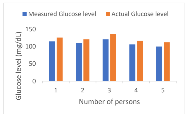
Figure 10. Glucose level of different persons measured after 3 hours of food using IR sensor and standard glucometer.
